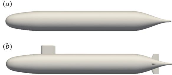
**Figure 1:** Depiction of the axisymmetric bare hull DARPA SUBOFF (a) and the appended DARPA SUBOFF (b).
